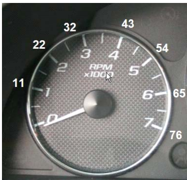
Figure 4: A tachometer displaying the number of human-days of air consumed by a 3.5 L engine as a function of rpm. Driving at 2000 rpm for one hour uses 22 human-days of air through the engine and converts that air into exhaust.
